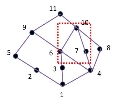
The upper bounds of B are 10, 11, and LUB(B) is 10 (the first vertex that can be Reached from {6,7,10} by upward paths )
