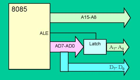
Given that ALE operates as a pulse during T1, we will be able to latch the address. Then when ALE goes low, the address is saved and the AD7– AD0 lines can be used for their purpose as the bi-directional data lines.
