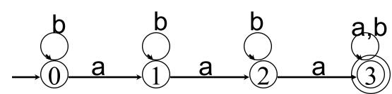
state-transition diagram for  $M_1$  note: the naming of states is not necessary
