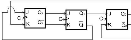
The above synchronous sequential circuit built using JK flip-flops is initialized with  $Q_2Q_1Q_0 = 000$ . The state sequence for this circuit for the next 3 clock cycles is
