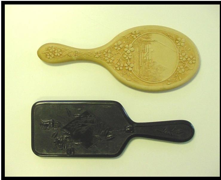
Molded plastic mirror frames and a hand made compression mold. (circa 1866)
