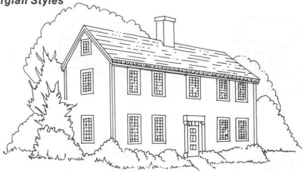
Side-gabled Roof, Cornice, and Central Chimney
