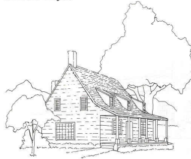
Dormers and Flared Roof
