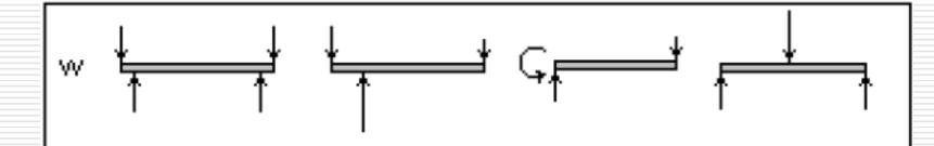
simple bending cantilever cantilever central load
