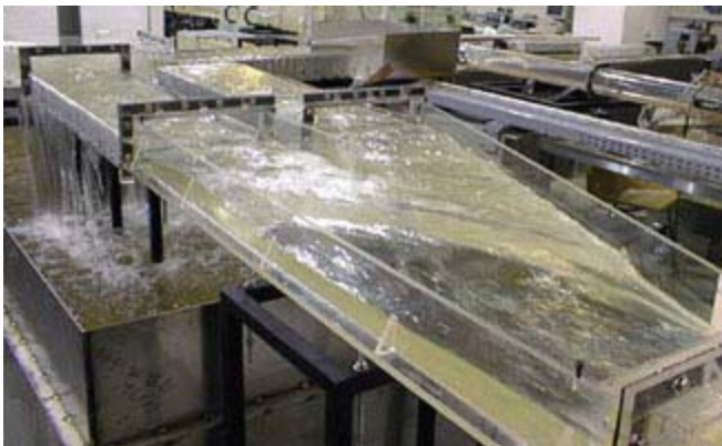
Scale model of side weir (1:22)
