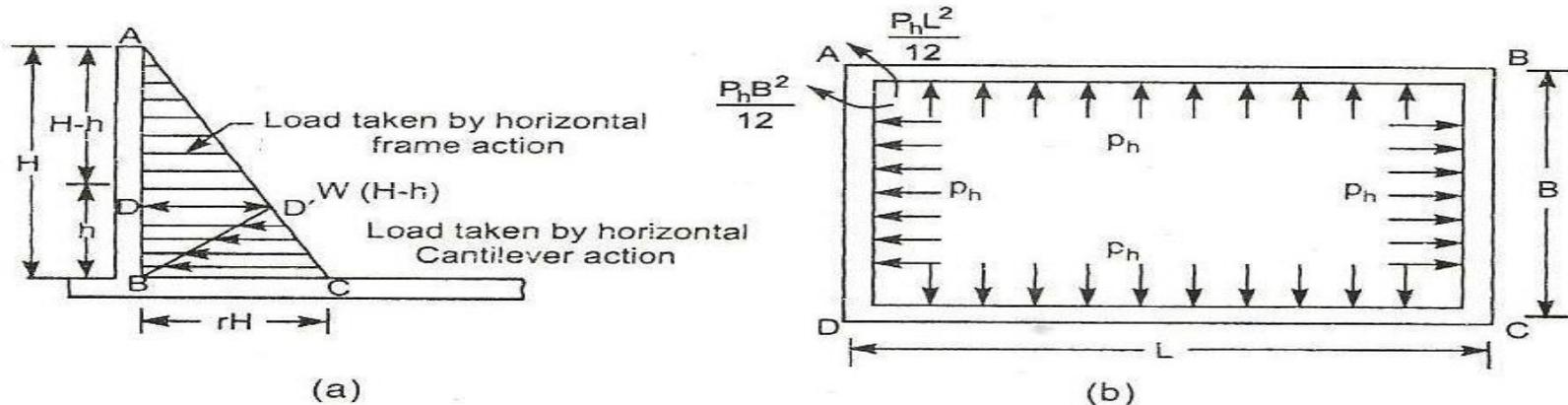
Fig. 13.6 Pressure Diagram
