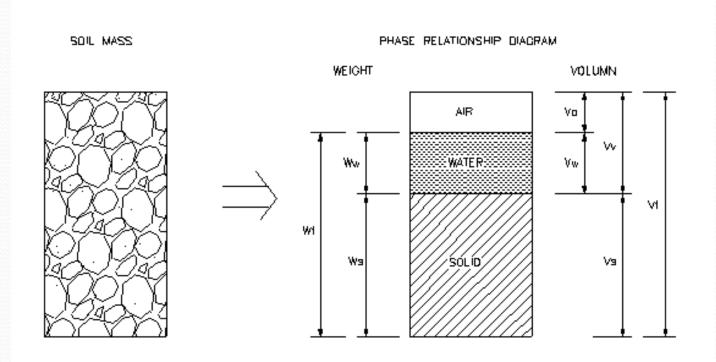
• If we determine the proportions of the components, we can calculate MANY other properties of the soil!
