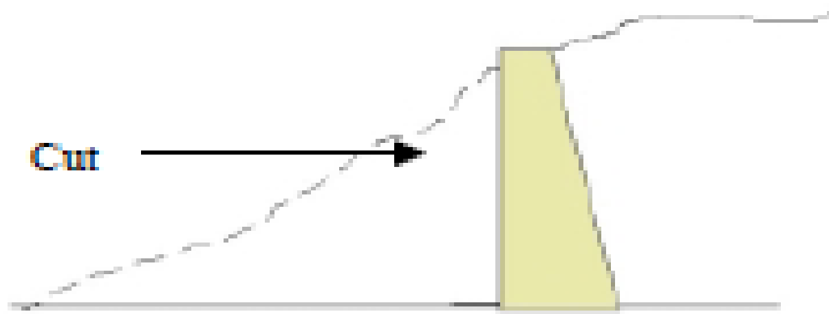
Retaining Wall to Support a Cut.
