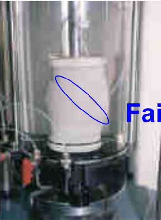
Soil sample at failure
