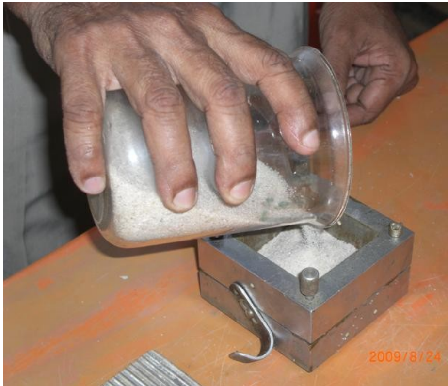
Preparation of a sand specimen
