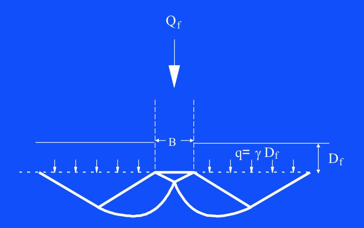
Mechanism analysed by Terzaghi
