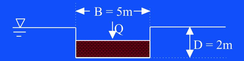
Determine short term and long term ultimate capacity given  $c_u = 25 \text{ kN/m}^2$ ,  $\phi_u = 0$ ,  $c' = 2 \text{ kN/m}^2$ ,  $\phi' = 25^\circ$ , and  $\gamma_{\text{sat}} = 15 \text{ kN/m}^2$ .
