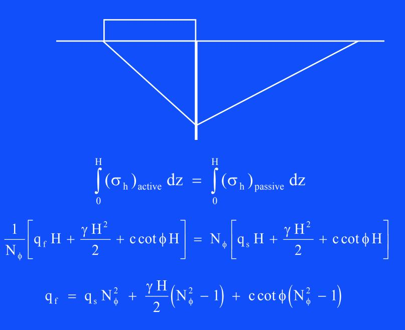
$$q_{f} = q_{s} N_{\phi}^{2} + \frac{\gamma H}{2} (N_{\phi}^{2} - 1) + c \cot \phi (N_{\phi}^{2} - 1)$$
