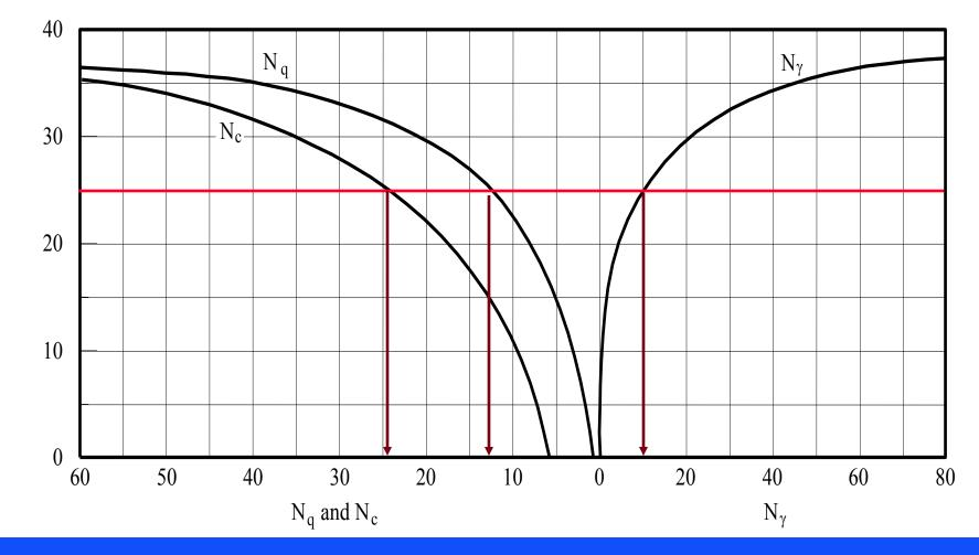
24.5 = and N<sub>c</sub>10 = , N<sub> $\gamma$ </sub>13 = N<sub>q</sub>25 = ' $\phi$
