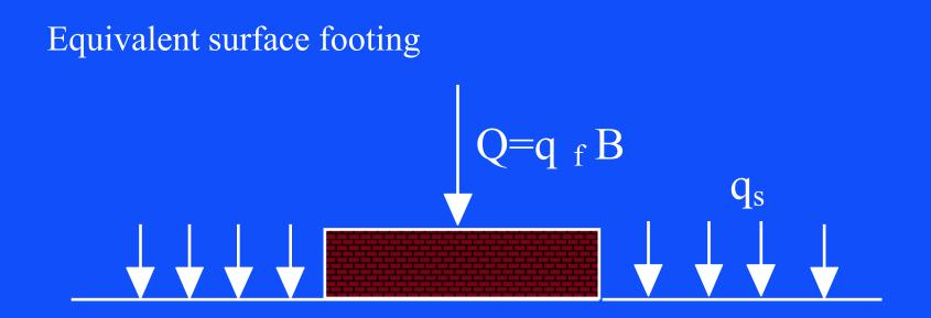
Short term - Undrained (total stress) analysis Position of water table not important - soil must be saturated  $q_s = \gamma_{sat} D = 15 \times 2 = 30 \text{ kPa}$
