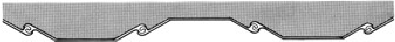
STEEL SHEET PILING
