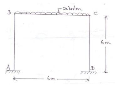
40) Analyze the frame shown in figure by the matrix stiffness method.
