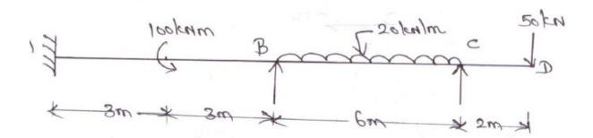
**35)** Analyze the continuous beam shown in figure by stiffness method. Draw the bending moment diagram.
