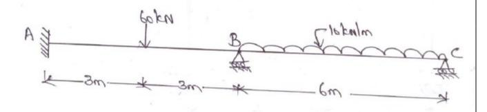
**33)** Analyze the continuous beam shown in figure .Assume EI as uniform. Use Matrix flexibility method.
