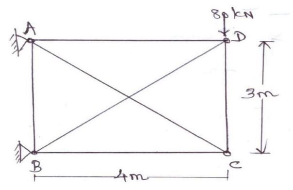
**31)** Analyze the truss loaded as shown in the figure using matrix flexibility method and find the member forces. A and E are the same for all members.
