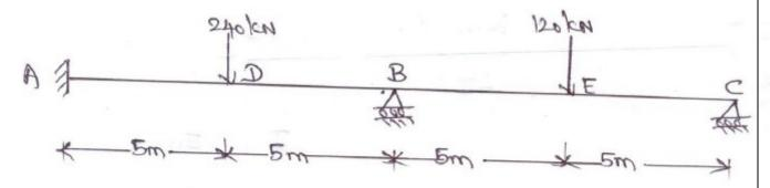
**34)** Analyze the continuous beam shown in figure .Assume EI as uniform. Use Matrix flexibility method.
