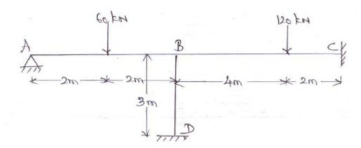
**40)** Analyze the frame shown in figure by the matrix stiffness method.
