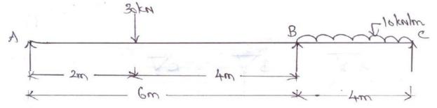
**30)** Analyze the frame shown in the figure by the matrix flexibility method.
