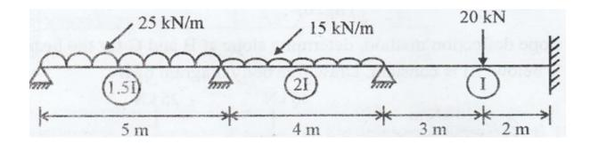
**43)** Analyze the Continuous beam shown in Fig. 10 using flexibility method and draw
