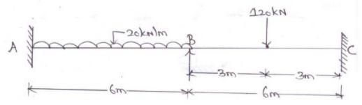
**36)** A two span continuous beam ABC is fixed at A and simply supported over the supports Band C. AB=6m and BC=6m. The moments of inertia is constant throughout. It is loaded as shown in the diagram. Analyse the beam by matrix stiffness method.
