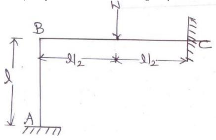
**39)** Analyze the frame shown in figure by the matrix stiffness method.
