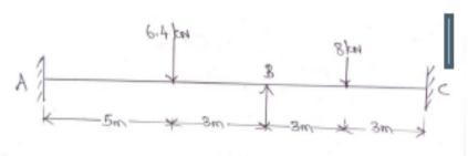
**38)** Analyze the structure shown in figure by stiffness method.
