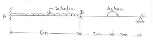
**37)** Analyze the continuous beam by matrix stiffness method
