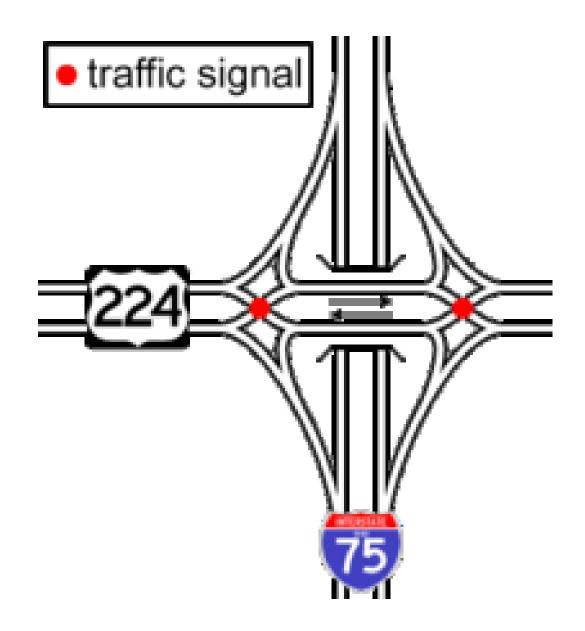
• The diverging diamond interchange allows for two-phase operation at all signalized intersections within the interchange.
