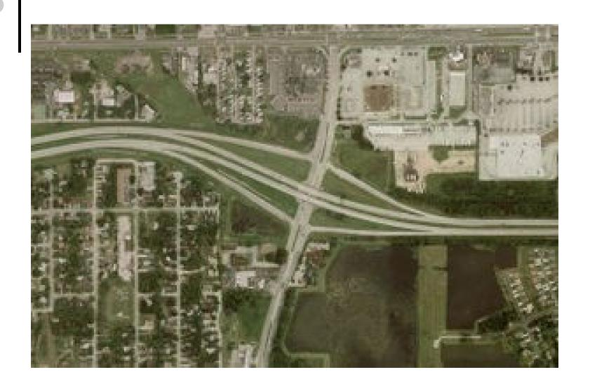
The diamond interchange makes more efficient use of space than most types of highway interchange, and avoids the interweaving traffic flows that occur in interchanges such as the cloverleaf.
