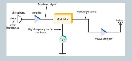
Figure 1: Modulation at the transmitter.
