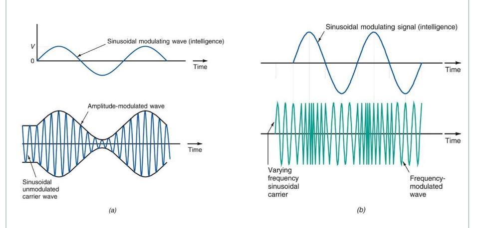
Figure 2: Types of modulation. (a) Amplitude modulation. (b) Frequency modulation.
