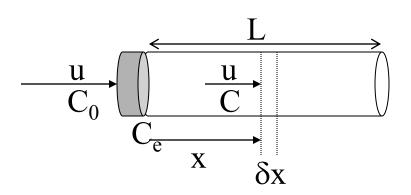
The concentraion will vary in the entry section due to diffusion, but will not vary in the section following the reactor. (Wehner and Wilhelm, 1956)
