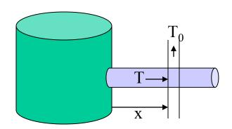
The sectional area of the electrode  $A = 1/4 \pi \times 0.15^2 = 0.0177 \text{ m}^2$ A heat balance over the length of electrode  $\delta x$  at distance x from the furnace is input - output = accumulation
