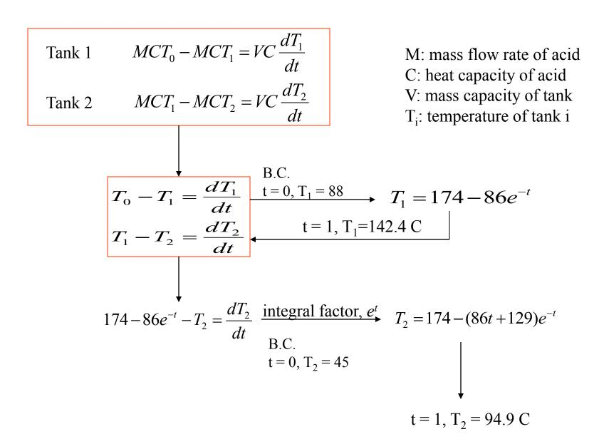
When water supply restores after 1 hour, heat balance for tank 1 and tank 2:
