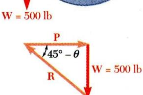
horizontally to the right, impending motion is clockwise to raise load. Utilize a force triangle to find *P*.
