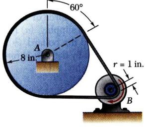
A flat belt connects pulley *A* to pulley *B*. The coefficients of friction are  $\mu_s = 0.25$ and  $\mu_k = 0.20$  between both pulleys and the belt.
