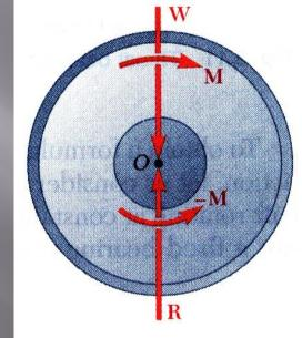
• Angle between *R* and normal to bearing surface is the angle of kinetic friction  $\varphi_k$ .
