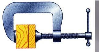
A clamp is used to hold two pieces of wood together as shown. The clamp has a double square thread of mean diameter equal to 10 mm with a pitch of 2 mm. The coefficient of friction between threads is  $\mu_s = 0.30$ .
