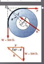
With the load on the left and force *P* acting horizontally to the right, impending motion is clockwise to raise load. Utilize a force triangle to find *P*.
