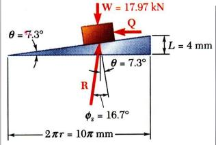
With impending motion down the plane, calculate the force and torque required to loosen the clamp.
