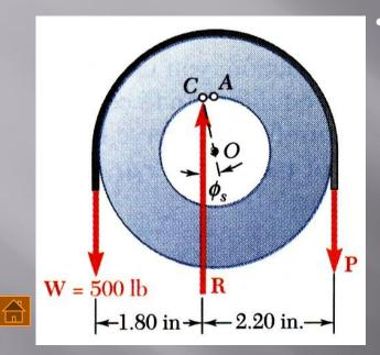
• Impending motion is counter-clockwise as load is held stationary with smallest force *P*. Sum moments about *C* to find *P*.
