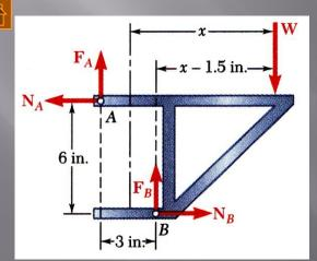
• When *W* is placed at minimum *x*, the bracket is about to slip and friction forces in upper and lower collars are at maximum value.
