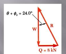
• Calculate lead angle and pitch angle. For the double threaded screw, the lead *L* is equal to twice the pitch.
