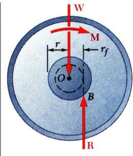
• For graphical solution, *R* must be tangent to *circle of friction*.
