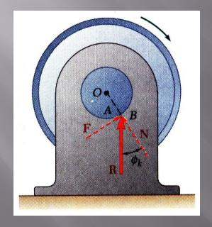
Journal bearings provide lateral support to rotating shafts. Thrust bearings provide axial support
