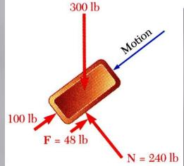
force required for equilibrium, block will slide. Calculate kinetic-friction force.
