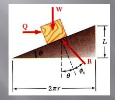
• Impending motion upwards. Solve for *Q*.
