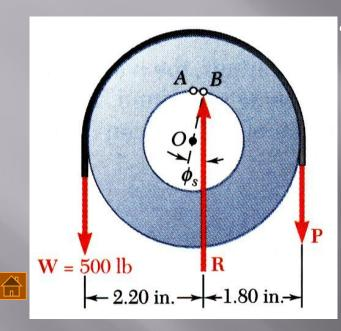
With the load on the left and force *P* on the right, impending motion is clockwise to raise load. Sum moments about displaced contact point *B* to find *P*.
