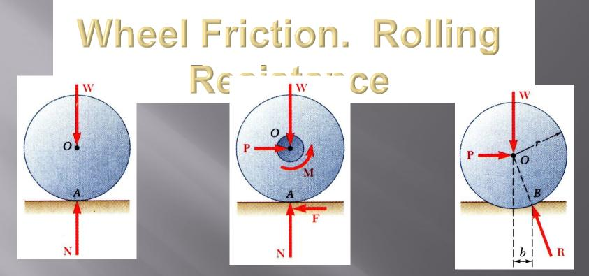
• Point of wheel in contact with ground has no relative motion with respect to ground.
