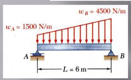
A beam supports a distributed load as shown. Determine the equivalent concentrated load and the reactions at the supports.
