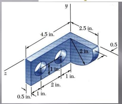
Locate the center of gravity of the steel machine element. The diameter of each hole is 1 in.
