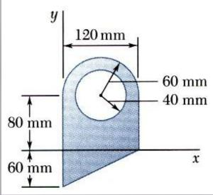
For the plane area shown, determine the first moments with respect to the x and y axes and the location of the centroid.
