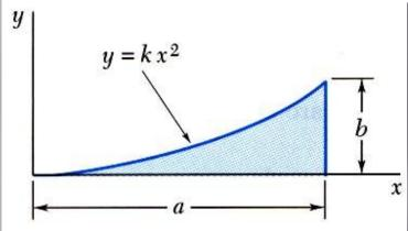
Determine by direct integration the location of the centroid of a parabolic spandrel.
