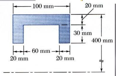
The outside diameter of a pulley is 0.8 m, and the cross section of its rim is as shown. Knowing that the pulley is made of steel and that the density of steel is  $\rho = 7.85 \times 10^3 \text{ kg/m}^3$  determine the mass and weight of the rim.
