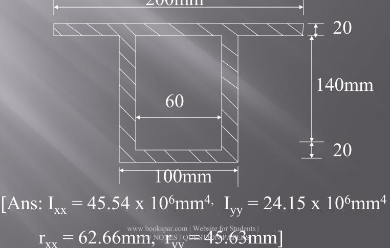
Q.4. Determine the horizontal and vertical centroidal M.I. Of the shaded portion of the figure.
