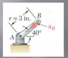
$\omega_{AB} = 2000 \text{ rpm} = 209.4 \text{ rad/s} = \text{constant}$   $\alpha_{AB} = 0$   $a_B = r \omega_{AB}^2 = \left(\frac{3}{12} \text{ ft}\right)(209.4 \text{ rad/s})^2 = 10,962 \text{ ft/s}^2$  $\vec{a}_B = \left(10,962 \text{ ft/s}^2\right)(-\cos 40^\circ \vec{i} - \sin 40^\circ \vec{j})$
