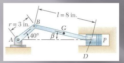
The crank *AB* has a constant clockwise angular velocity of 2000 rpm.
