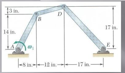
In the position shown, crank *AB* has a constant angular velocity  $\omega_1 = 20$  rad/s counterclockwise.
