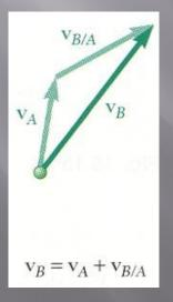
• Any plane motion can be replaced by a translation of an arbitrary reference point *A* and a simultaneous rotation about *A*.
