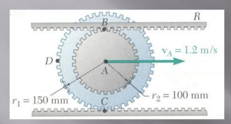
The double gear rolls on the stationary lower rack: the velocity of its center is 1.2 m/s.
