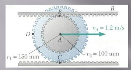
The double gear rolls on the stationary lower rack: the velocity of its center is 1.2 m/s.
