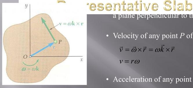
y  $a_i = \alpha k \times r$ P $a_n = -\omega^2 r$  $\omega = \omega k$  $\alpha = \alpha k$
