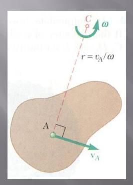
replaced by the translation of an arbitrary point A and a rotation about A with an angular velocity that is independent of the choice of A.
