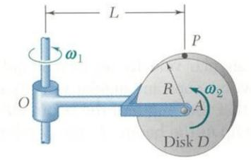
For the disk mounted on the arm, the indicated angular rotation rates are constant.
