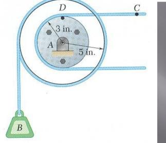
Cable *C* has a constant acceleration of 9  $in/s^2$  and an initial velocity of 12 in/s, both directed to the right.
