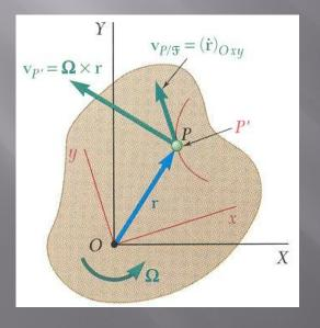
• Frame OAT is fixed and frame OAY foraces with angular velocity  $\vec{\Omega}$ .
