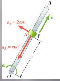
relative velocity u along rod OB. The rod is rotating at a constant angular velocity  $\omega$ . The point A on the rod corresponds to the instantaneous position of P.
