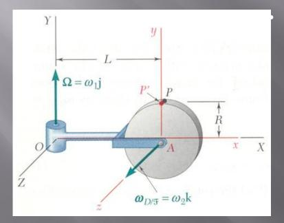
With *P*' of the moving reference frame coinciding with *P*, the velocity of the point *P* is found from  $\vec{v}_P = \vec{v}_{P'} + \vec{v}_{P/F}$  $\vec{v}_{P'} = \vec{\Omega} \times \vec{r} = \omega_1 \vec{j} \times (L\vec{i} + R\vec{j}) = -\omega_1 L \vec{k}$  $\vec{v}_{P/F} = \vec{\omega}_{D/F} \times \vec{r}_{P/A} = \omega_2 \vec{k} \times R\vec{j} = -\omega_2 R \vec{i}$  $\vec{v}_P = -\omega_2 R \vec{i} - \omega_1 L \vec{k}$
