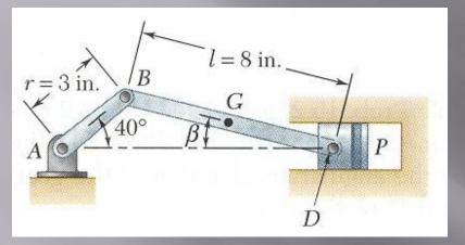
Crank *AG* of the engine system has a constant clockwise angular velocity of 2000 rpm.
