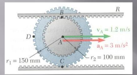
The center of the double gear has a velocity and acceleration to the right of 1.2 m/s and 3 m/s<sup>2</sup>, respectively. The lower rack is stationary.
