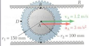
• The expression of the gear position as a function of  $\theta$  is differentiated twice to define the relationship between the translational and angular accelerations.
