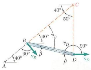
$\gamma_B = 40^\circ + \beta = 53.95^\circ$  $\gamma_D = 90^\circ - \beta = 76.05^\circ$
