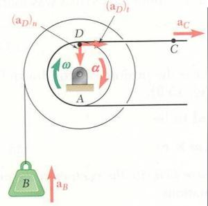
For the life in target for and normal acceleration components of *D*.  $(\vec{a}_D)_t = \vec{a}_C = 9 \text{ in./s} \rightarrow$  $(a_D)_n = r_D \omega_0^2 = (3 \text{ in.})(4 \text{ rad/s})^2 = 48 \text{ in/s}^2$  $(\vec{a}_D)_t = 9 \text{ in./s}^2 \rightarrow (\vec{a}_D)_n = 48 \text{ in./s}^2 \downarrow$
