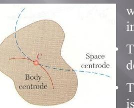
• The particle coinciding with the center of rotation changes with time and the acceleration of the particle at the instantaneous center of rotation is not zero.
