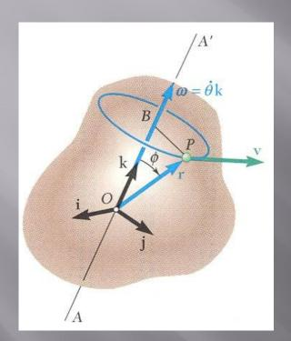
• Motion of a rigid body rotating around a fixed axis is often specified by the type of angular acceleration.
