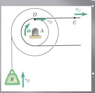
The tangential velocity and acceleration of D are equal to the velocity and acceleration of C.
