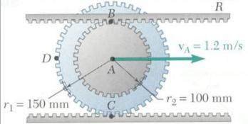
The displacement of the gear center in one revolution is equal to the outer circumference.
