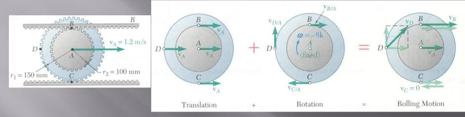
Velocity of the upper rack is equal to velocity of point *B*:
