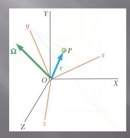
• The absolute acceleration can be expressed as  $\vec{a}_P = \vec{\Omega} \times \vec{r} + \vec{\Omega} \times (\vec{\Omega} \times \vec{r}) + 2\vec{\Omega} \times (\vec{r})_{Oxyz} + (\vec{r})_{Oxyz}$  $= \vec{a}_{p'} + \vec{a}_{P/F} + \vec{a}_c$
