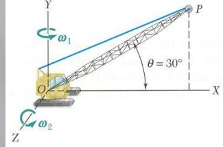
The crane rotates with a constant angular velocity  $\omega_1 = 0.30$  rad/s and the boom is being raised with a constant angular velocity  $\omega_2 = 0.50$  rad/s. The length of the boom is l = 12 m.
