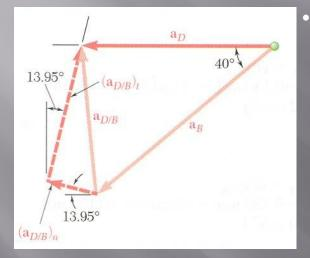
Component equations for acceleration of point *D* are solved simultaneously.
