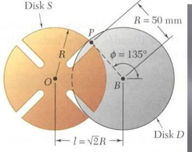
In the Geneva mechanism, disk *D* rotates with a constant counterclockwise angular velocity of 10 rad/s. At the instant when  $\varphi = 150^{\circ}$ , determine angular acceleration of disk *S*. • The absolute acceleration of the pin *P* may be expressed as
