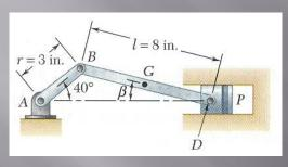
The directions of the accelerations  $\vec{a}_D$ ,  $(\vec{a}_{D/B})_t$ , and  $(\vec{a}_{D/B})_n$  are determined from the geometry.
