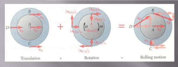
The acceleration of each point is obtained by adding the acceleration of the gear center and the relative accelerations with respect to the center.
