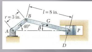
• The angular acceleration of the connecting rod *BD* and the acceleration of point *D* will be determined from
