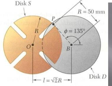
Disk D of the Geneva mechanism rotates with constant counterclockwise angular velocity  $\omega_D = 10$  rad/s.
