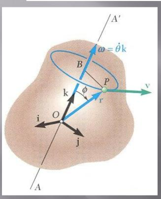
$$\vec{a} = \frac{d\vec{v}}{dt} = \frac{d}{dt} (\vec{\omega} \times \vec{r})$$
