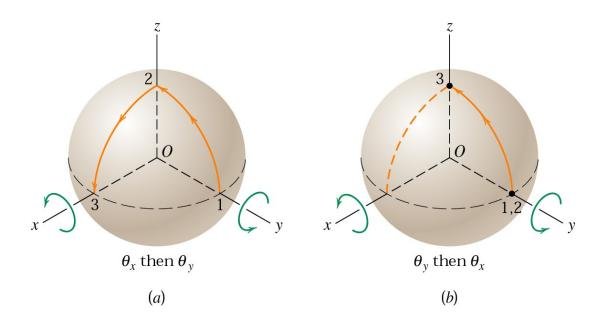
On the other hand, if the order of the rotations is reversed, the point undergoes no motion during the y-rotation but moves to point 3 during the 90° rotation about x-axis. Thus, the two cases do not produce the same final position, and it is evident from this one special example that finite rotations do not generally obey the parallelogram law of vector addition and are not commutative. (a+b $\neq$ b+a)
