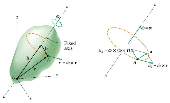
Any point such as A which is not on the axis moves in a circular arc in a plane normal to the axis and has a velocity and an acceleration
