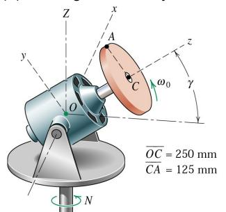
The rotor and disk have two components of angular velocity :  $\omega_o$ =120(2 $\pi$ )/60=4 $\pi$  rad/s about the z-axis and  $\Omega$ = 60(2 $\pi$ )/60=2 $\pi$  rad/s about the Z-axis.
