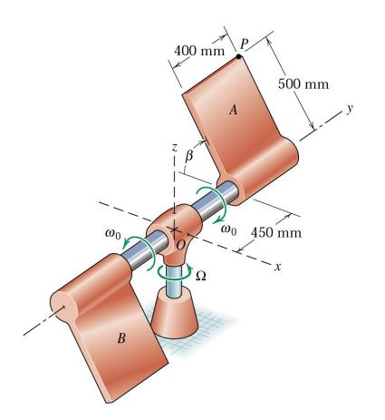
The panel assembly and attached x-y-z axes rotate with a constant angular velocity  $\Omega$ =0.6 rad/s about the vertical z-axis. Simultaneously, the panels rotate about the y-axis as shown with a constant  $\omega_0$ =2 rad/s. Determine the angular acceleration  $\alpha$  of panel A and find the acceleration of point P for the instant when  $\beta$ =90°.
