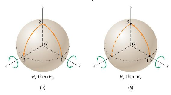
In part (a) of the figure, two successive 90° rotations of the sphere about, first, the x-axis and second, the y axis result in the motion of a point which is initially on the y-axis in position 1, to positions 2 and 3, successively.
