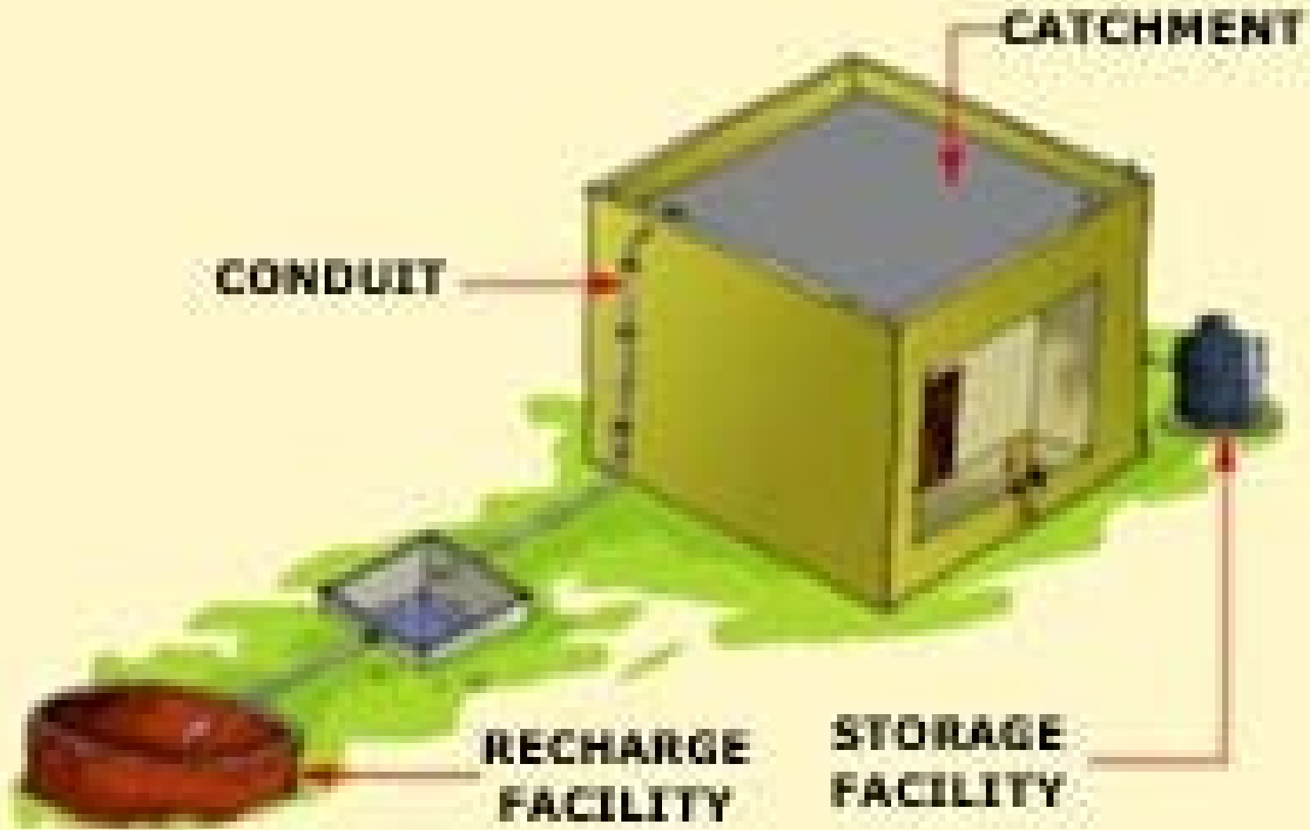
ELEMENTS OF A TYPICAL WATER HARVESTING SYSTEM
