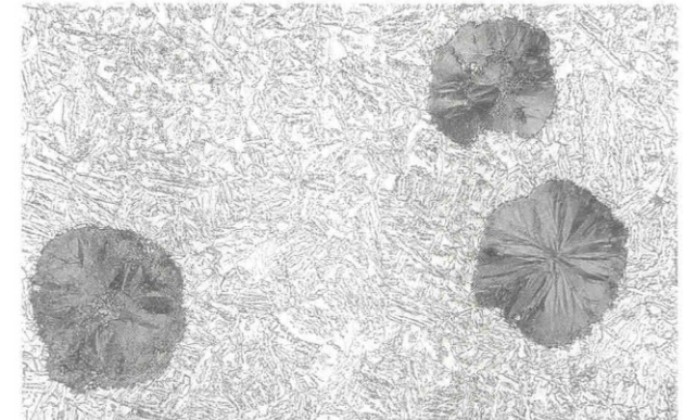
Fig. 2 Austempered ductile iron structure consisting of spheroidal graphite in a matrix of bainitic ferritic plates (dark) and interplate austenitic (white). The heat treat cycle was austenitized at 870^{\circ}\text{C} ( 1600^{\circ}\text{F} ) for 3 h followed by austempering at 385^{\circ}\text{C} ( 725^{\circ}\text{F} ) for 2 h. 500 \times . Courtesy of B.V. Kovacs, Kosmar Enterprises
