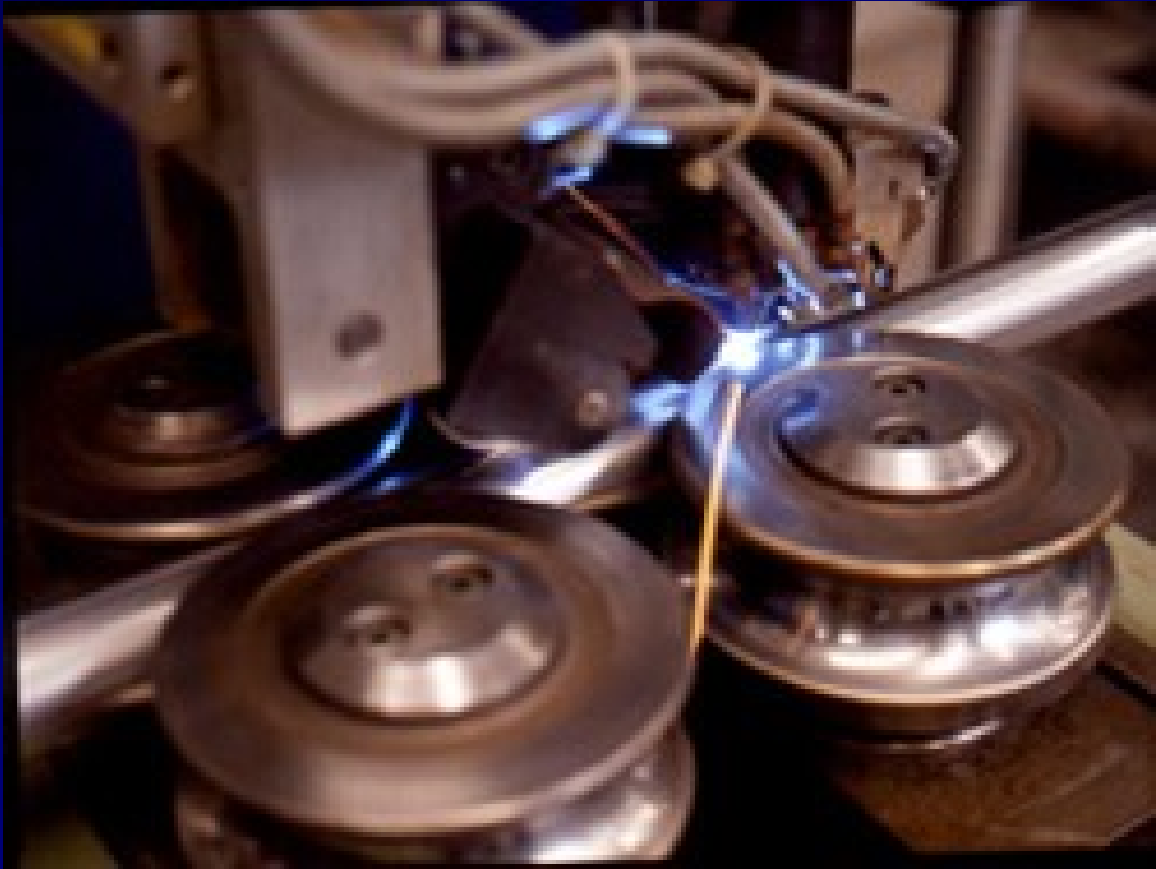
Laser welding of a pipe
