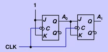
Example: 3-bit synchronous binary counter (using T flip-flops, or JK flip-flops with identical J, K inputs).
