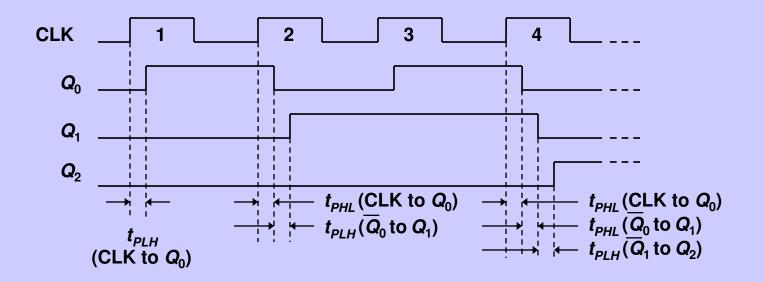
Example: 4-bit ripple binary counter (negative-edge triggered).
