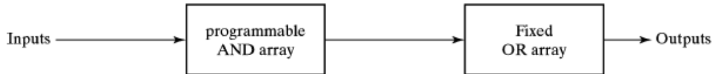
(b) Programmable array logic (PAL)
