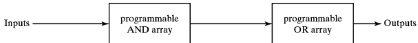
(c) Programmable logic array (PLA)
