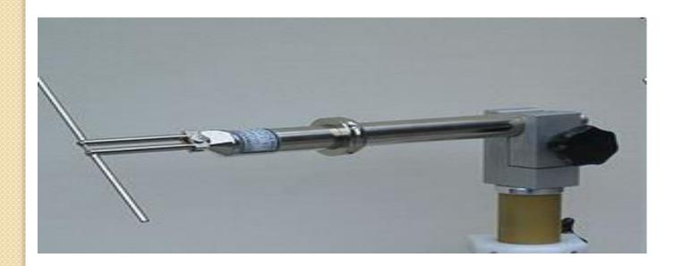
Dipoles have an radiation pattern, doughnut symmetrical about the axis of the dipole. The radiation is maximum at right angles to the dipole, dropping off to zero on the antenna's axis.
