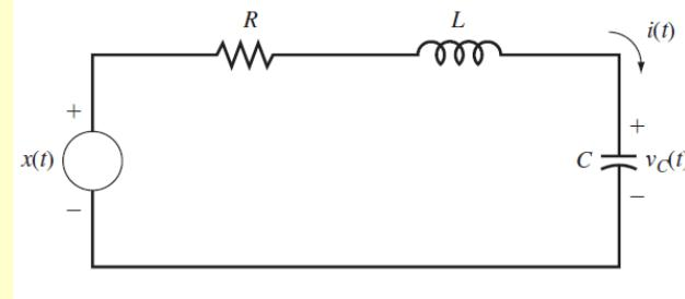
$$\frac{d^2 y(t)}{dt^2} + \left( \frac{R}{L} \right) \frac{dy(t)}{dt} + \frac{1}{LC} y(t) = \frac{1}{LC} x(t)$$
