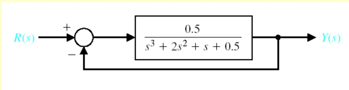
A closed-loop control system example for
