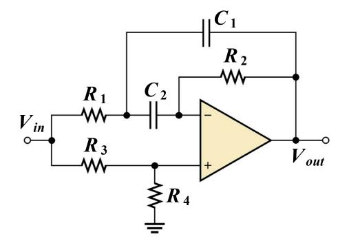
> The configuration is similar to the band-pass version BUT  $R_3$  has been moved and  $R_4$  has been added.
