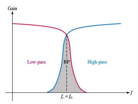
$\succ$  The band-pass output peaks sharply the center frequency giving it a high Q.
