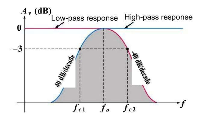
>The lower frequency  $f_{c1}$  of the passband is the critical frequency of the high-pass filter.
