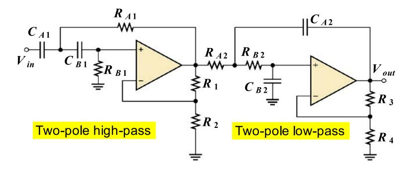
Band-pass filter is formed by cascading a two-pole high-pass and two pole low-pass filter.
