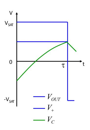
Half-cycle ends when  $V_C$  reaches  $V_{SAT}/2$
