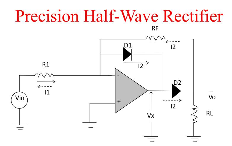
• Solid arrows represent current flow for positive half-cycles of  $V_{in}$  and dashed arrows represent current flow for negative half-cycles
