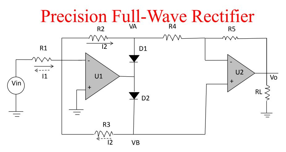
• Solid arrows represent current flow for positive half-cycles of  $V_{in}$  and dashed arrows represent current flow for negative half-cycles
