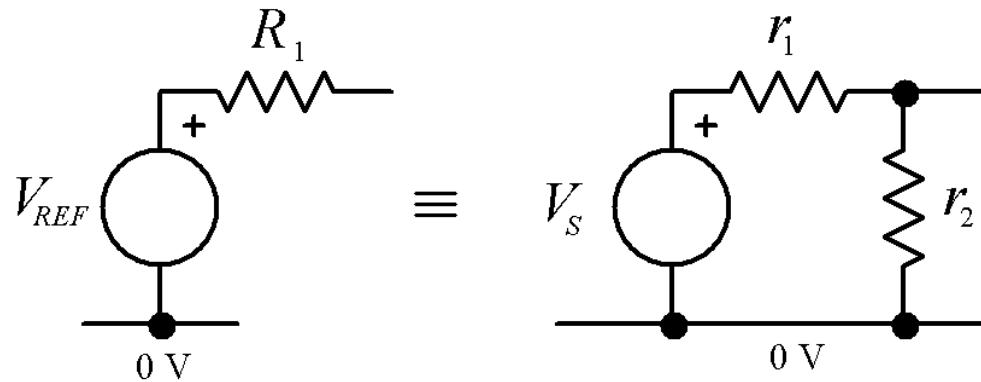
Providing  $R_1 = r_1 \parallel r_2$        $V_{REF} = V_S \frac{r_2}{r_1 + r_2}$
