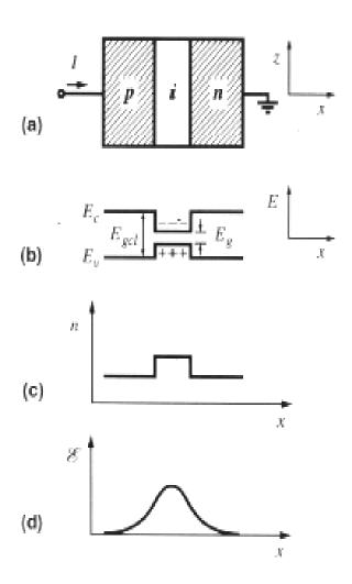
**Double Heterostructure** provides **transverse confinement** of both Carriers and Photons
