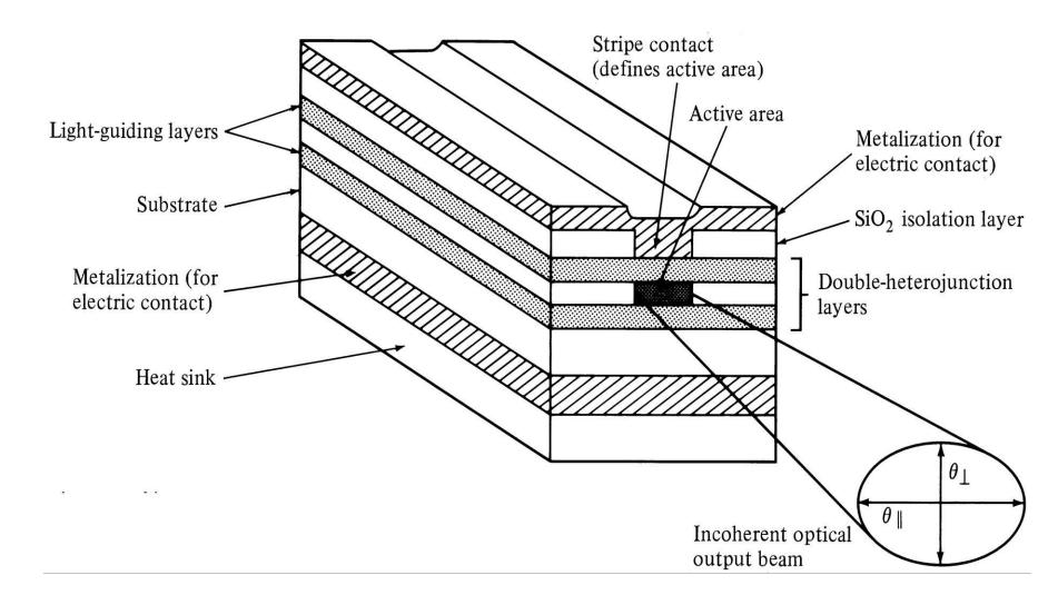
The active region is embedded into a waveguide structure so that the light is directed an edge
