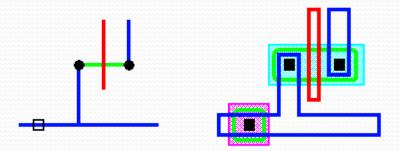
• An N-Well Tap is inferred where the connection is from a power rail while a Substrate Tap is inferred where the connection is from a ground rail.
