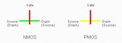
• There is no difference in the construction of a transistor source and a transistor drain. The source is determined as the source of conductors (electrons for NMOS / holes for PMOS) when current flows through the channel. In some pass transistor circuits, the source and drain may swap over during use.
