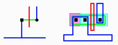
• A combined contact and tap can only be used where the end of a diffusion stick coincides with a contact to the power or ground rail.
