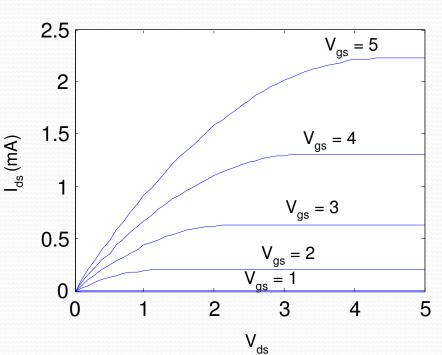
$$\beta = \mu C_{ox} \frac{W}{L} = (350) \left( \frac{3.9 \bullet 8.85 \cdot 10^{-14}}{100 \cdot 10^{-8}} \right) \left( \frac{W}{L} \right) = 120 \frac{W}{L} \mu A / V^2$$
