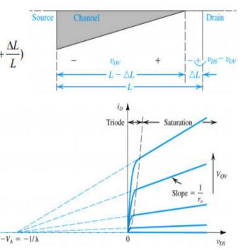
$\Box V_A$  (Early voltage) =  $1/\lambda$  is proportional to channel length:  $V_A = V'_A L$  $\Box V'_A$  is process-technology dependent with a typical value from 5 ~ 50 V/µm.
