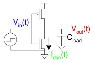
$$\begin{aligned} & V_{in}(t) = u(t - t_0)V_{DD} \\ & V_{out}(t < t_0) = \\ & \frac{dV_{out}(t)}{dt} = \end{aligned}$$
