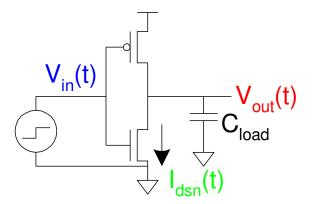
$$\begin{aligned} & V_{in}(t) = u(t - t_0)V_{DD} \\ & V_{out}(t < t_0) = V_{DD} \\ & \frac{dV_{out}(t)}{dt} = \end{aligned}$$
