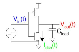
$$\begin{aligned} V_{in}(t) &= u(t - t_0)V_{DD} \\ V_{out}(t < t_0) &= V_{DD} \\ \frac{dV_{out}(t)}{dt} &= -\frac{I_{dsn}(t)}{C_{load}} \end{aligned}$$
