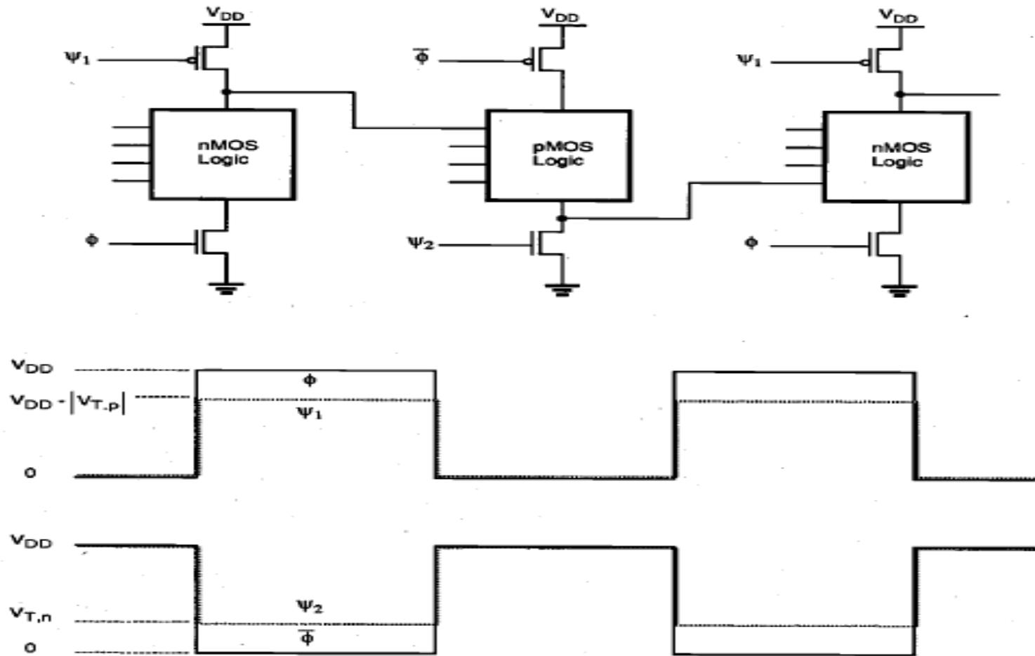
Fig. General circuit structure and the clock signals of Zipper CMOS
