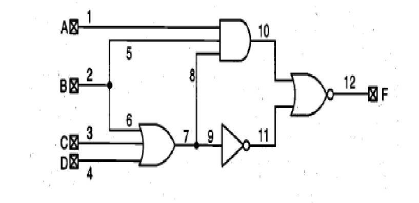
Fig. A simple circuit consisting of four gates with four primary inputs and one primary output.
