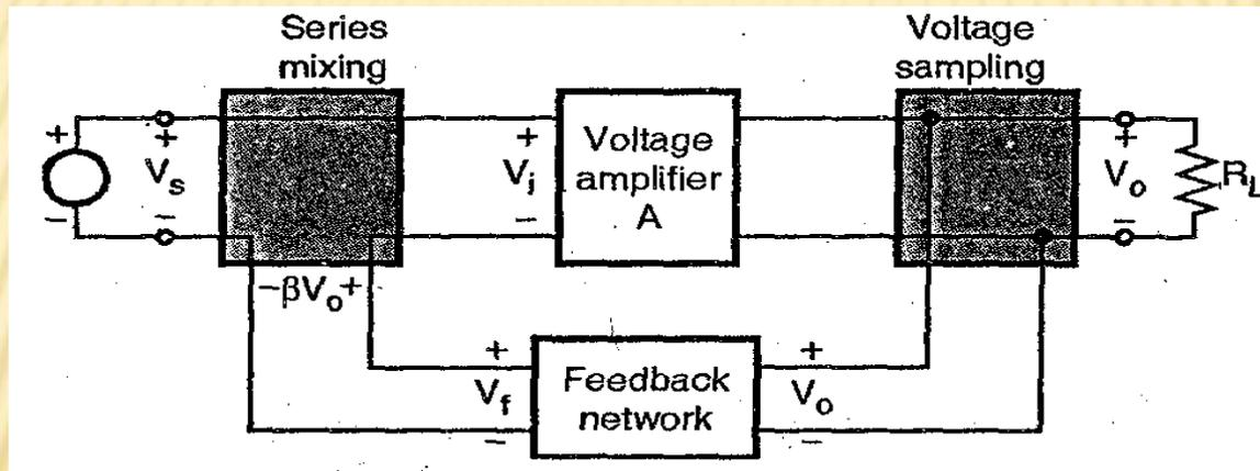
A transistor amplifier which uses the voltage series feedback is the common collector or emitter follower amplifier:
