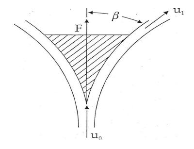
• Consider a vane symmetrical about the x-axis as shown in Figure 2.0. A jet of fluid flowing at the rate of (m dot) kg/s along the x-axis with the velocity  $u_0$  m/s strikes the vane and is deflected by it through angle  $\beta$ , so that the fluid leaves the vane with the velocity  $u_0$  m/s inclined at an angle  $\beta$  to the x-axis.
