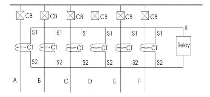
Here, in the figure above we assume that at normal condition feed, A, B, C, D, E & F carries current  $I_A$ ,  $I_B$ ,  $I_C$ ,  $I_D$ ,  $I_E$  and  $I_F$ . Now, according to Kirchoff's current law,
