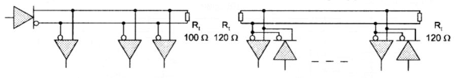
1 generator up to 10 receiver simplex operation
