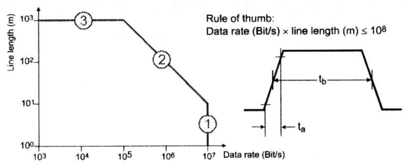
Data rate is limited by the rise time of the output signal of the generator (ITU-T V.11:  $t_r \le 0.1 \times t_b$ ; ISO8482:  $t_r \le 0.3 \times t_b$ ).
