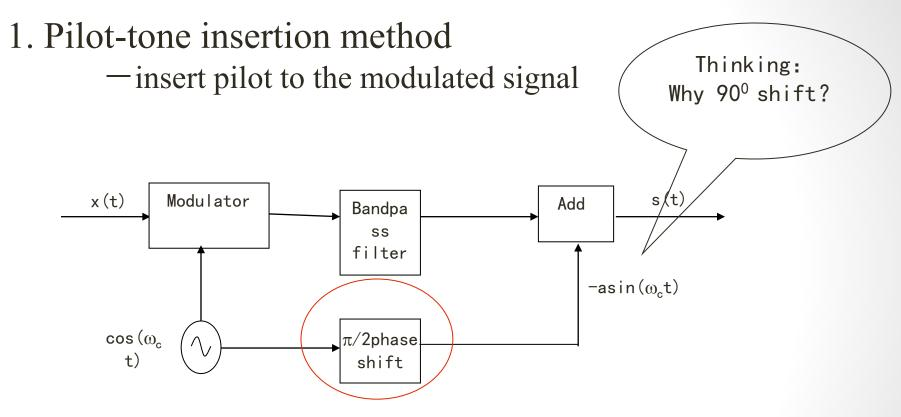
The pilot signal is generated by shift the carrier by  $90^{0}$  and decrease by several dB, then add to the modulated signal. Assume the modulated signal has 0 DC component, then the pilot is
