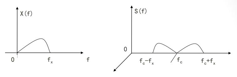
The receiver uses a narrowband filter with central frequency  $f_c$  to extract the pilot  $a \sin \omega_c t$  and then the carrier  $a \cos \omega_c t$  can be generated by simply shifting 90<sup>0</sup>.
