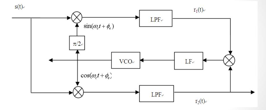
Contains in-phase branch and orthogonal branch. All parts except LF and VCO are similar with a "phase detector".
