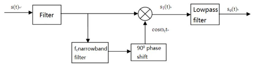
$$s_{1}(t) = s(t) \cdot \cos \omega_{c} t = f(t) \cos^{2} \omega_{c} t - a \sin \omega_{c} t \cos \omega_{c} t$$
