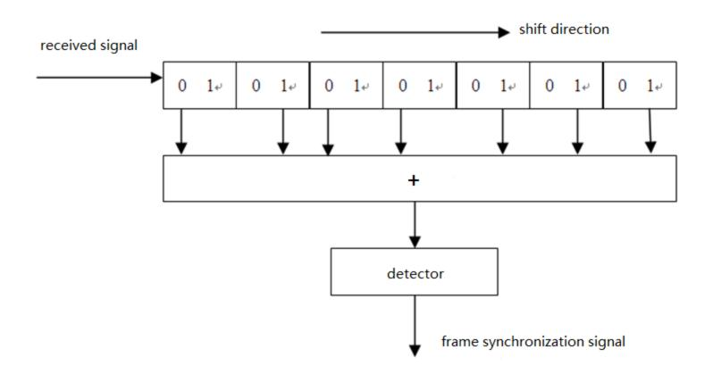
The barker code detector follows: input:"1" {output "1":? +1 output "0":? -1 input:"0" {output "1":? -1 output "0":? +1
