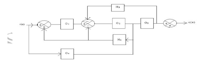
Q.7 For the system represented by the block diagram shown in fig. Determine C1/R1 and C2/R1.
