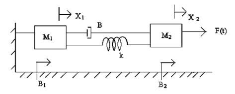
Q.3 Determine the transfer function Y2(S)/F(S) of the system shown in fig.
