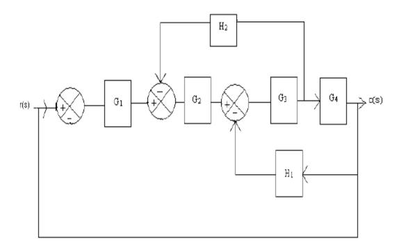
Q.6 Obtain the closed loop transfer function C(S)/R(S) of the system whose block diagram is shown in fig.
